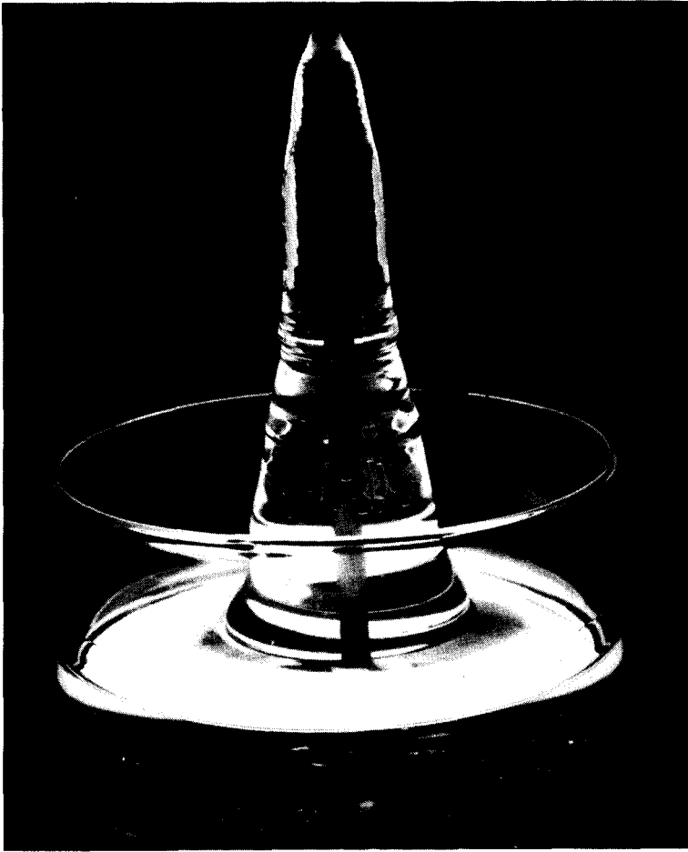
Fig. 4.7 The Weissenberg effect shown by a solution of polyisobutylene (Oppanol B200) in polybutene (B.P. Hyvis 07). Reproduced by permission of Shell Research Ltd.
